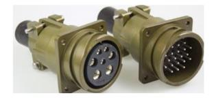
MG 00 wall mounting receptacles are used to carry wires through walls or bulkheads or to provide a means of disconnection at a Bulkhead. MG 00 receptacles mate with MG 06 and MG 08 style cable mount connectors.
